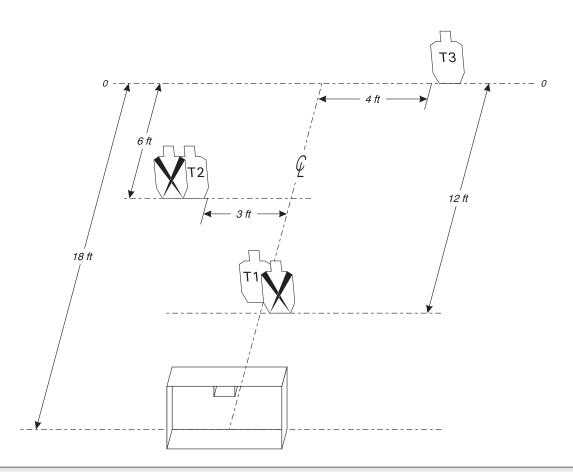
**SETUP NOTES:** Set paper targets to 5 feet high at shoulders. The "counter" can consist of saw horses. The shelf can be an opened cardboard box nailed to the underside of planking or boards. Have a replacement handy. Counter is 4 feet high by 8 feet wide by 2 feet deep.
